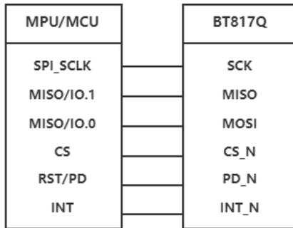
Figure 6. QSPI interface connection
