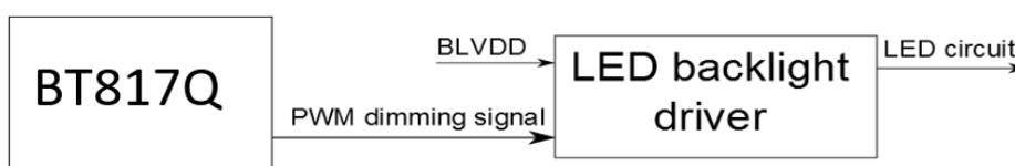
The LED backlight driver used in this module does not burst the LED current. Therefore, it does not generate audible noises on the output capacitor. It is equipped with soft start subsystem, which increases LED lifetime, as LED current peaks are reduced significantly.
