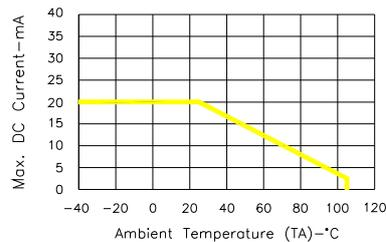
Fig.7-Max. Allowable DC Current
