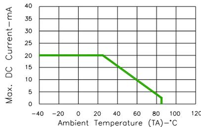
Fig.7-Max. Allowable DC Current
