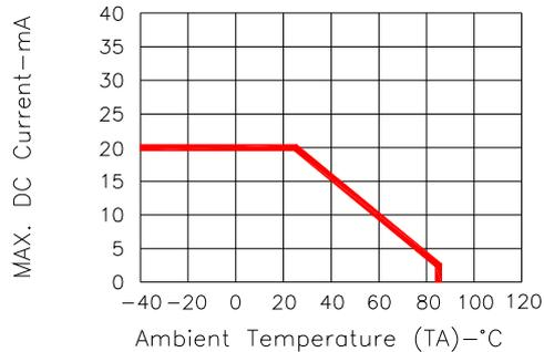
Fig.6 MAX. ALLOWABLE DC CURRENT VS. AMBIENT TEMPERATURE
