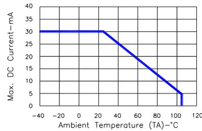
Fig.7-Max. Allowable DC Current
