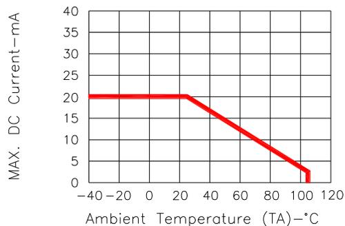
Fig.6 MAX. ALLOWABLE DC CURRENT VS. AMBIENT TEMPERATURE
