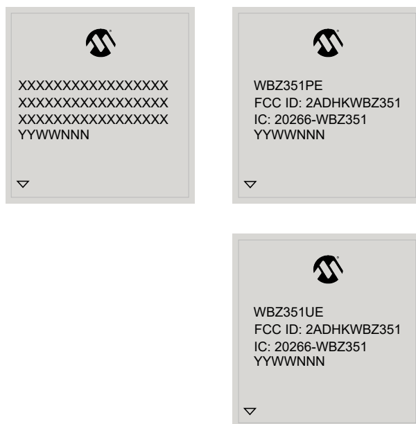
Figure 44-3. WBZ35x Module Packaging Marking
