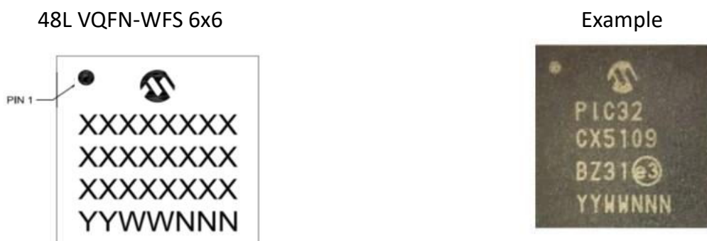
Figure 44-1. PIC32CX5109BZ31048/PIC32CX5109BZ36048 Package Marking
