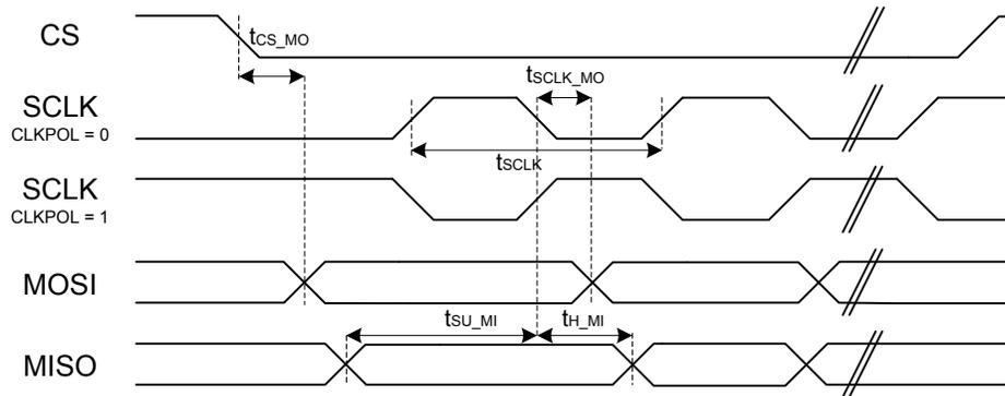
Figure 4.4. SPI Main Timing (SMSDELAY = 1)
