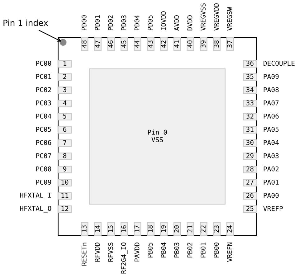
Figure 6.4. QFN48 / Standard Device Pinout
