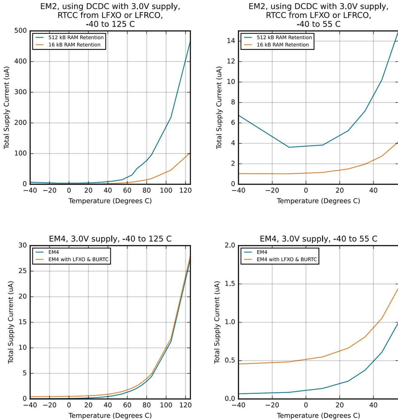
**Figure 4.10. EM2 and EM4 Typical Supply Current vs. Temperature**
