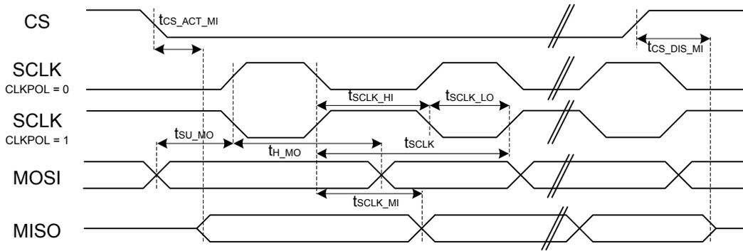
Figure 4.5. SPI Secondary Timing (SSSEARLY = 0)
