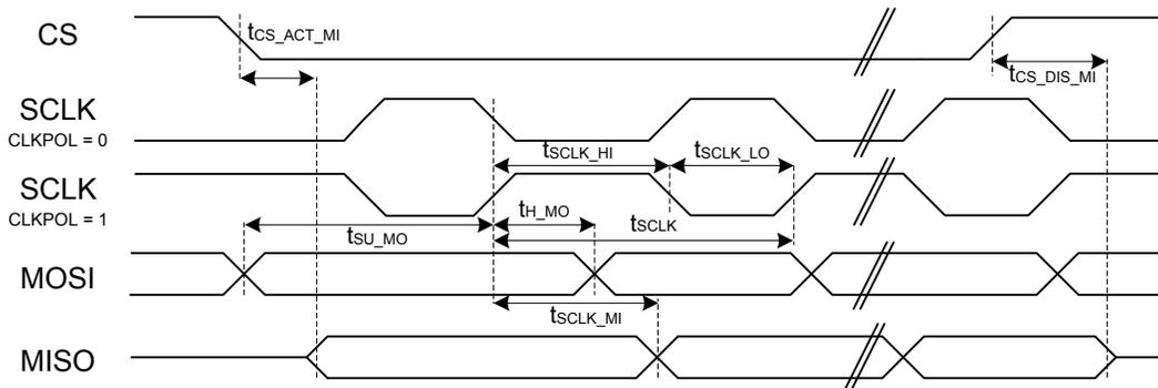
Figure 4.6. SPI Secondary Timing (SSSEARLY = 1)
