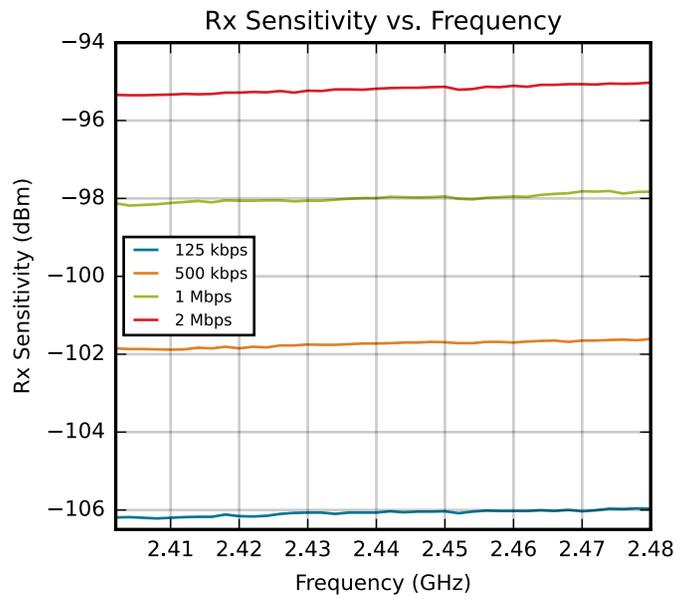
Figure 4.15. 2.4 GHz BLE RF Receiver Sensitivity
