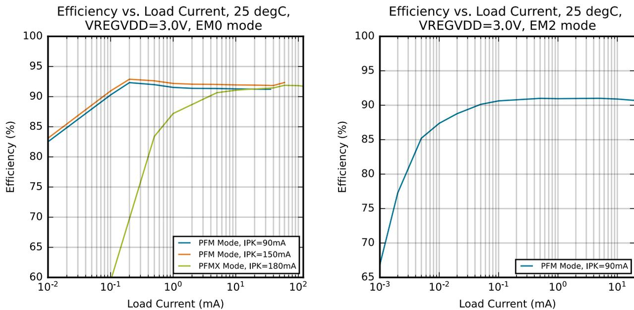
Figure 4.16. DC-DC Efficiency
