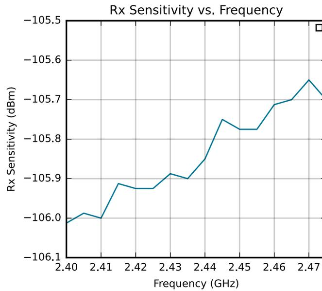
Figure 4.14. 2.4 GHz 802.15.4 RF Receiver Sensitivity
