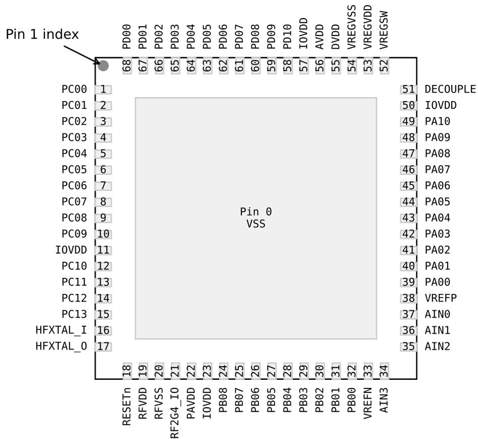
Figure 6.3. QFN68 / ADC Device Pinout
