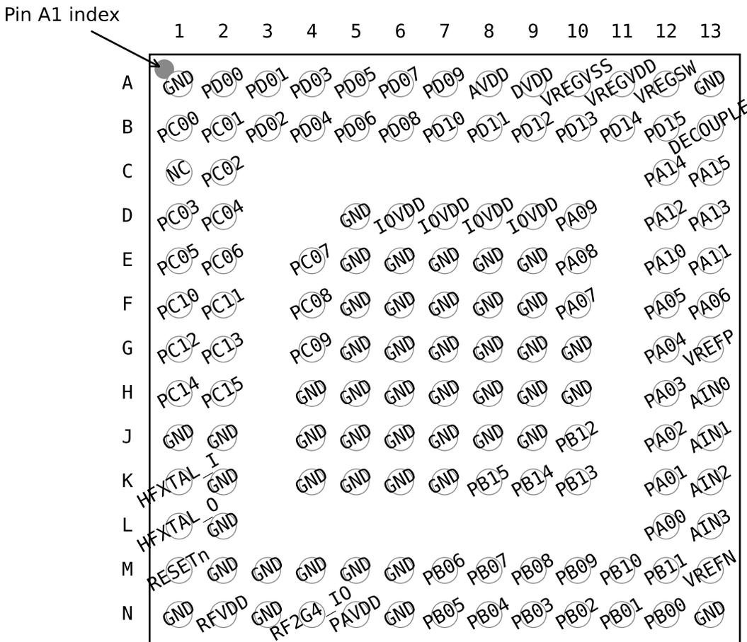
Figure 6.1. BGA136 / ADC Device Pinout
