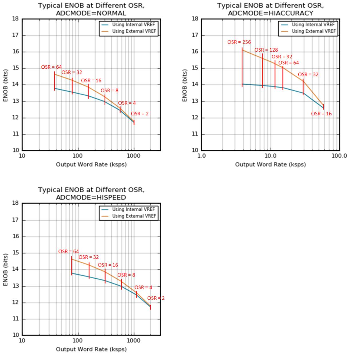
Figure 4.17. Typical ENOB vs. Oversampling Ratio
