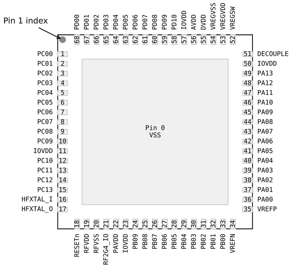
Figure 6.2. QFN68 / Standard Device Pinout
