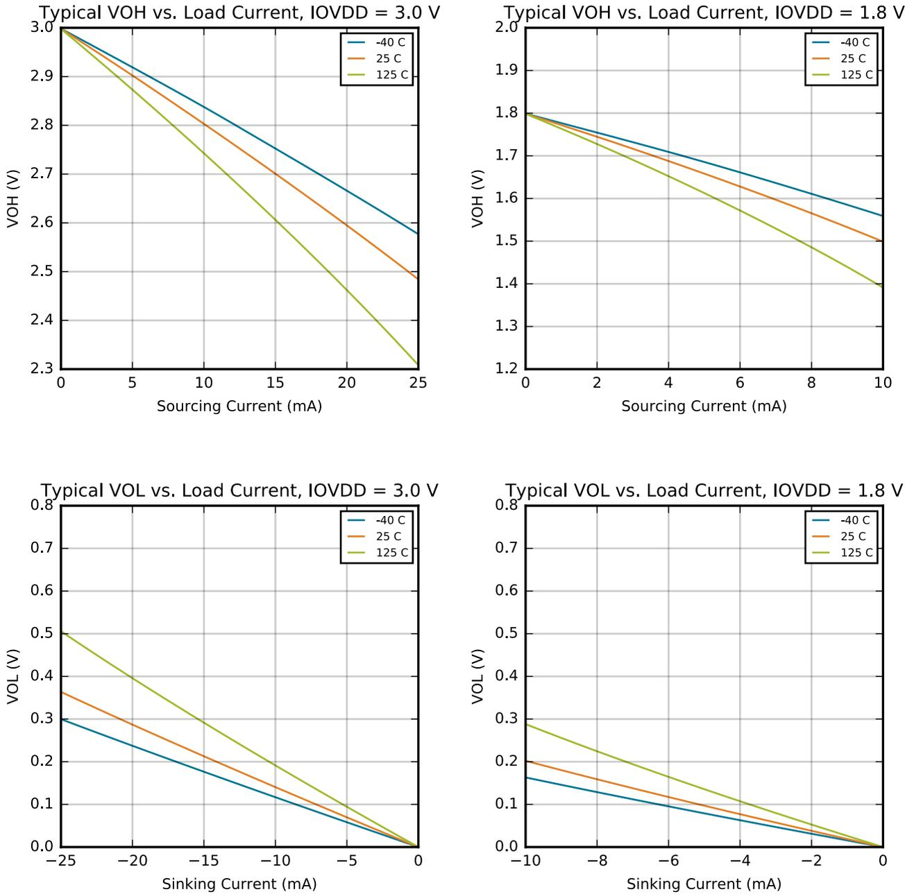
Figure 4.18. VOH and VOL vs. Load Current
