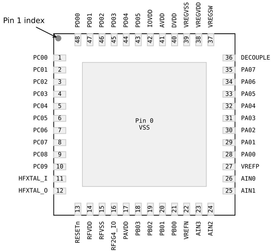
Figure 6.5. QFN48 / ADC Device Pinout
