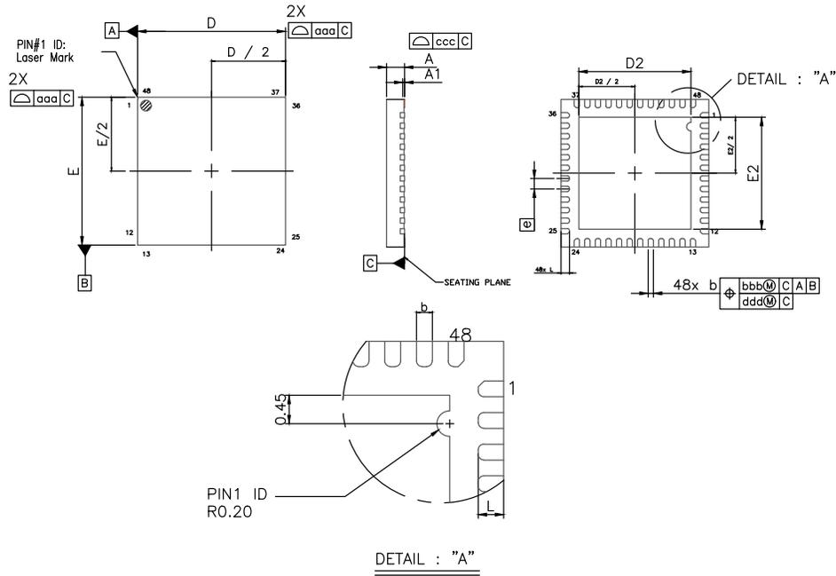
Figure 2. 7x7 mm 48-Pin QFN Package Diagram
