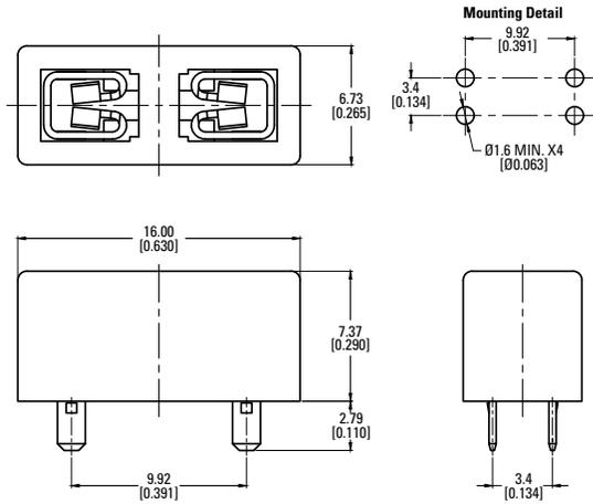
**01000065Z For Mini Fuse Surface Mount Installation**
