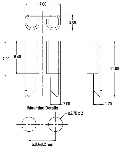
**01000062Z Low Profile Fuse Block for Type C or ATFO blade fuses**
