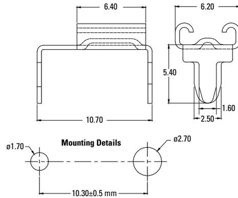
**01000061Z Vertical Fuse Clip for Type C or ATFO blade fuses**
