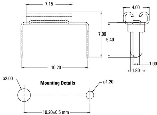
**01000060Z Horizontal Fuse Clip for Type C or ATFO blade fuses**
