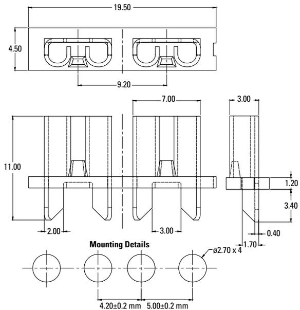
**01000063Z Low Profile Fuse Block for Type F or MINI blade fuses**
