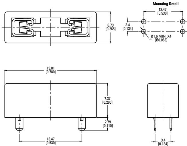
**01000067Z For Mini And ATO Fuse Through Hole Installation**
