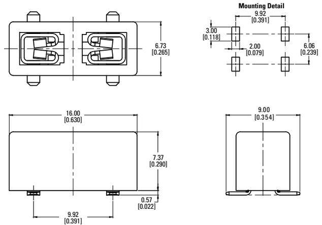
**01000066Z For ATO Fuse Through Hole Installation**
