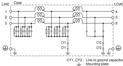
(2) Line to ground capacitor code : 355
