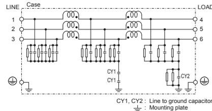
(3) Line to ground capacitor code : 203, 693, 104, 324
