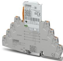
Surge protection, consisting of protective plug and base element, with integrated status indicator for a 4-wire floating signal circuit with high nominal current. Ideal for 4-wire measurements, e.g., of temperatures and weights. Can be used in safety-related circuits up to SIL 3.
