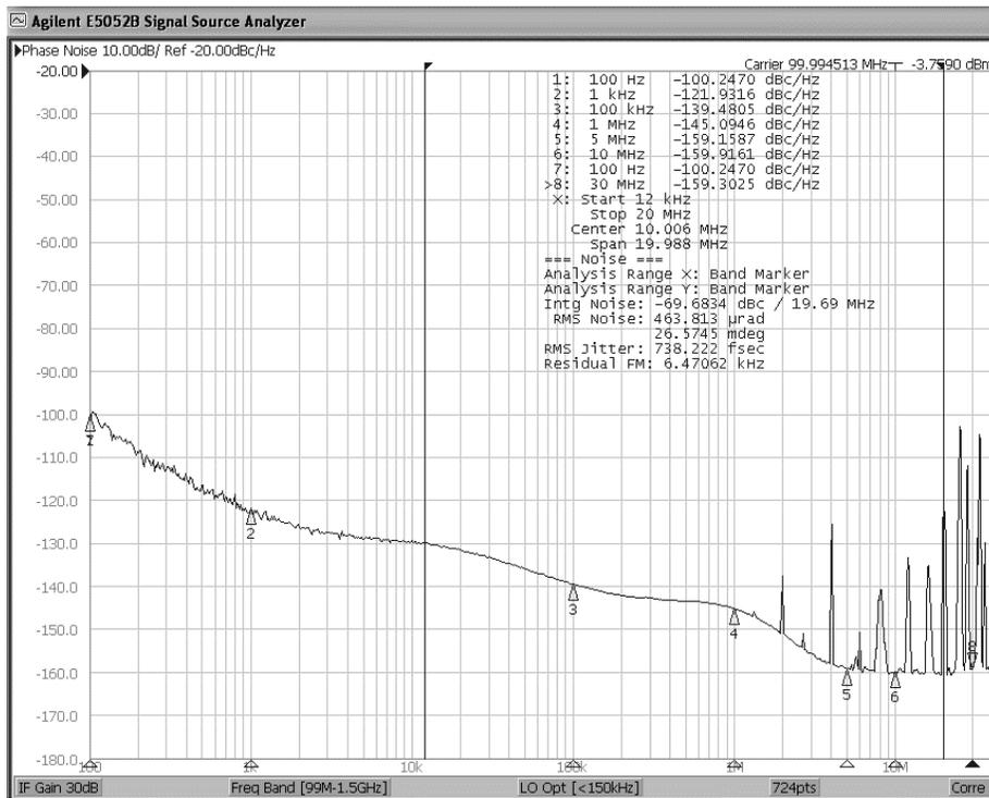
**100MHz LVDS: 0.74ps Phase Jitter for 12KHz to 20MHz**
