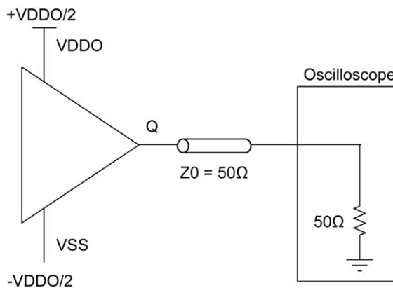
Figure 5. LVC MOS Output Load and Test Circuit
