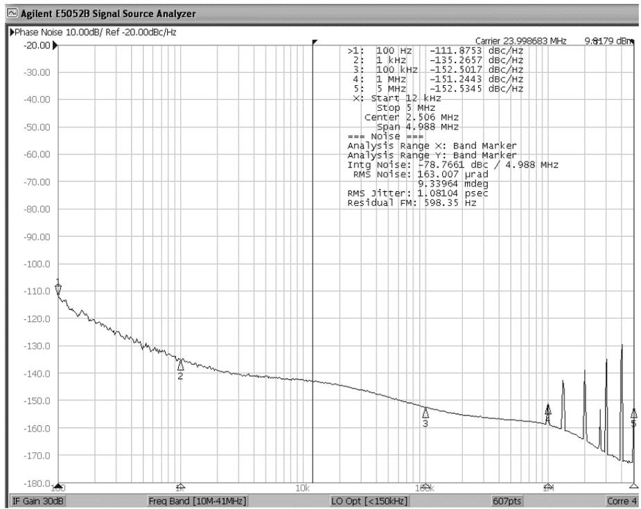
**24MHz LVC MOS: 1.1ps Phase Jitter for 12KHz to 5MHz**
