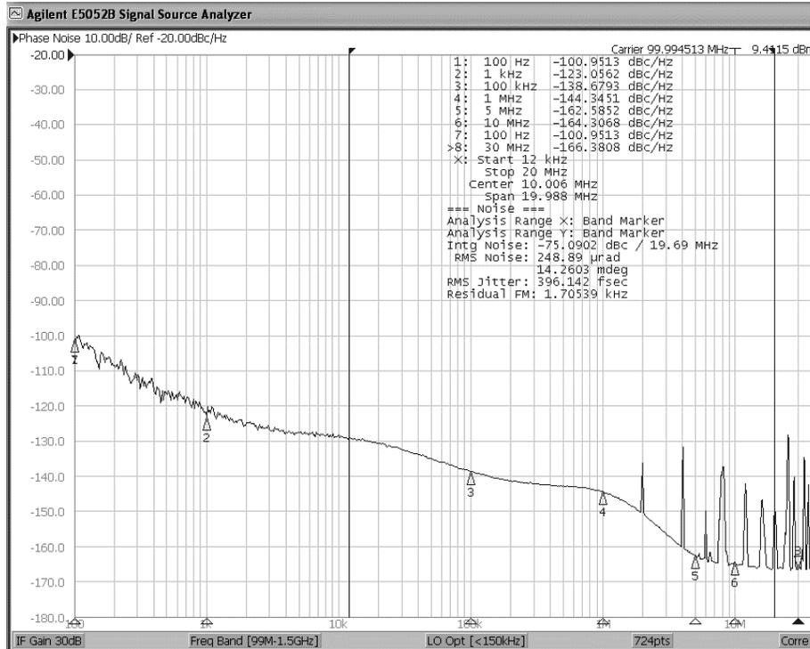
**100MHz LVC MOS: 0.40ps Phase Jitter for 12KHz to 20MHz**
