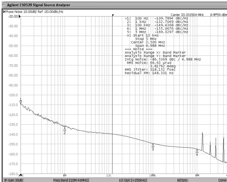
**33.33MHz LVC MOS: 0.32ps Phase Jitter for 12KHz to 5MHz**
