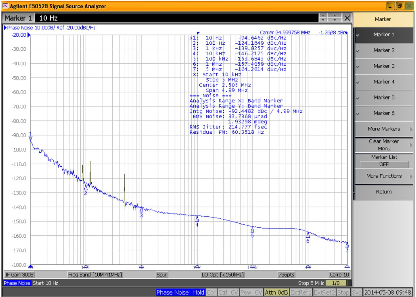
25MHz LVDS: 0.21ps Phase Jitter for 10KHz to 5MHz
