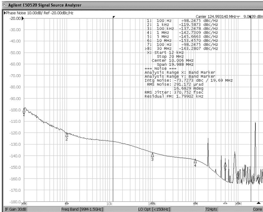
**125MHz LVC MOS: 0.37ps Phase Jitter for 12KHz to 20MHz**
