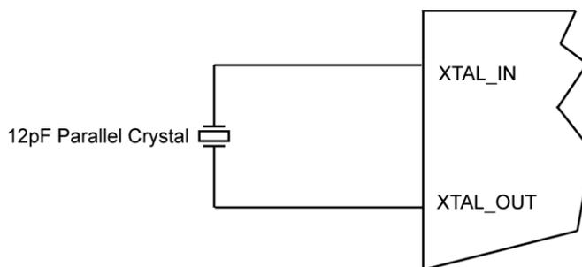
Figure 6. Crystal Input Interface
