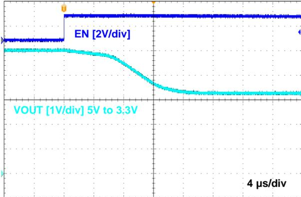
**Figure 21. V<sub>OUT</sub> Switchover from 5 V to 3.3 V**
