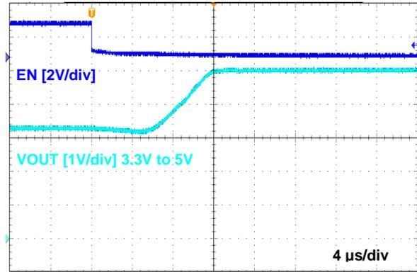
**Figure 21. V<sub>OUT</sub> Switchover from 3.3 V to 5 V**
