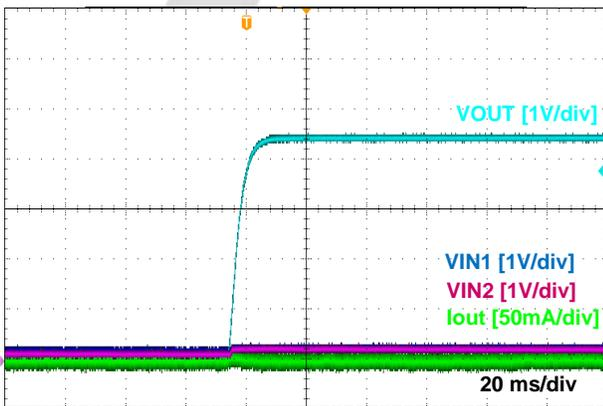
**Figure 23. Reverse Current Blocking When Disabled**
