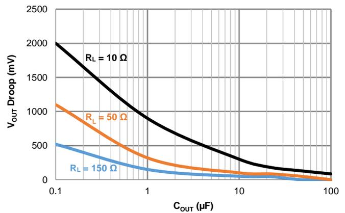
**Figure 25. Output Voltage Droop at Switching Over from V<sub>IN2</sub> (3.3 V) to V<sub>IN1</sub> (5 V)**
