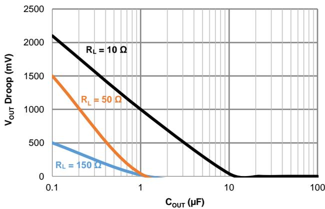
**Figure 24. Output Voltage Droop at Switching Over from V<sub>IN1</sub> (5 V) to V<sub>IN2</sub> (3.3 V)**
