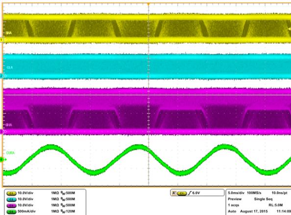
Figure 22. Motor Spinning 1000 RPM
