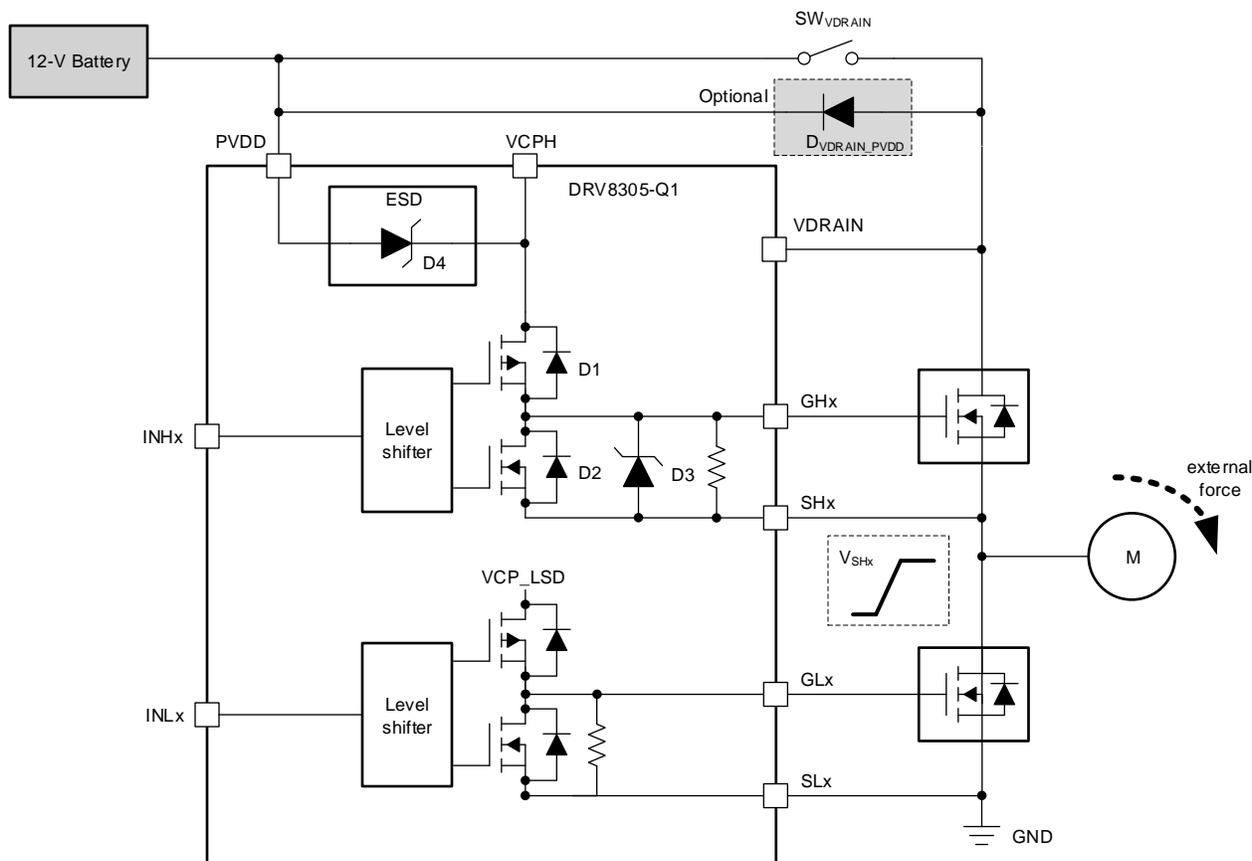
Figure 24. Power Supply Consideration in Generator Mode
