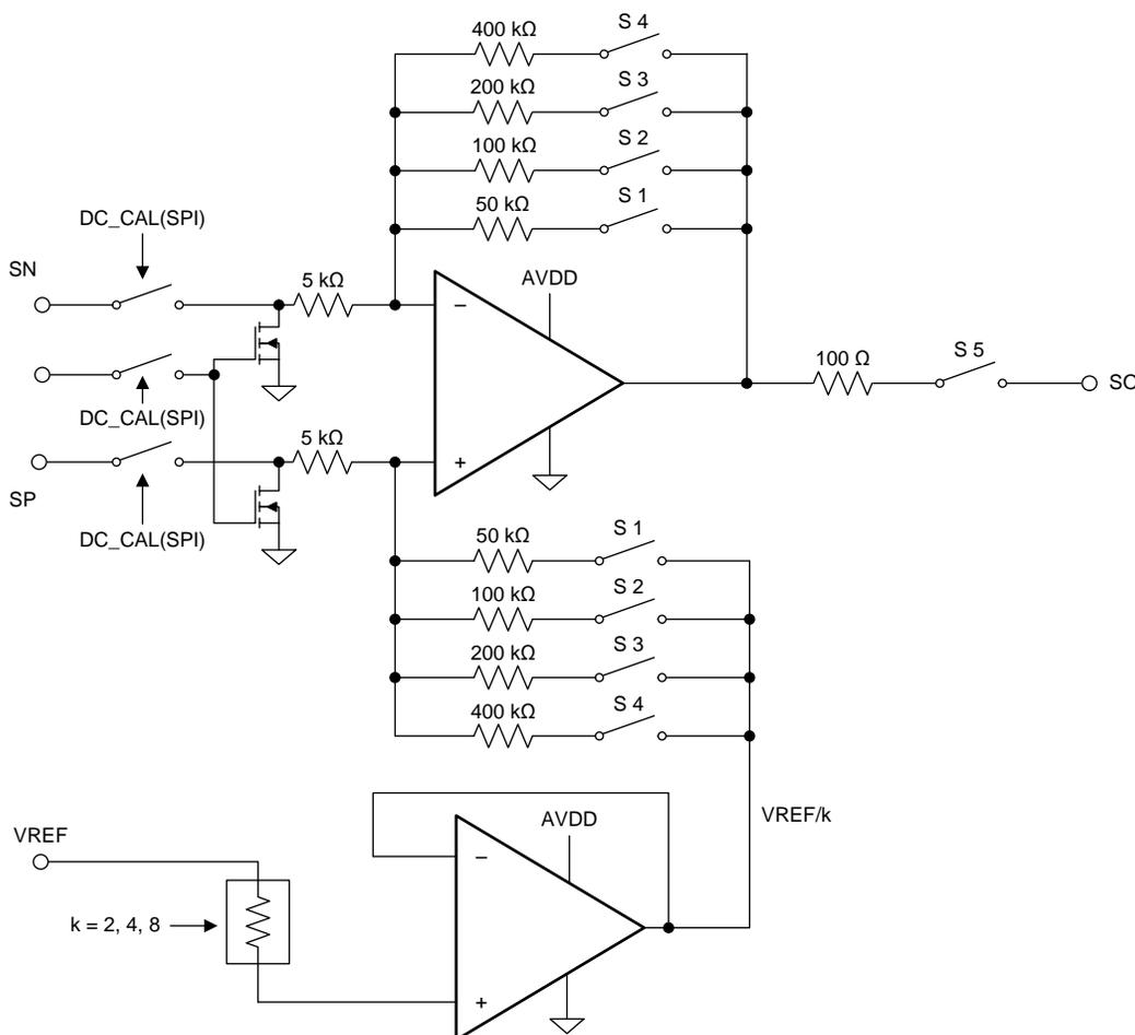
Figure 12. Current Shunt Amplifier Simplified Block Diagram
