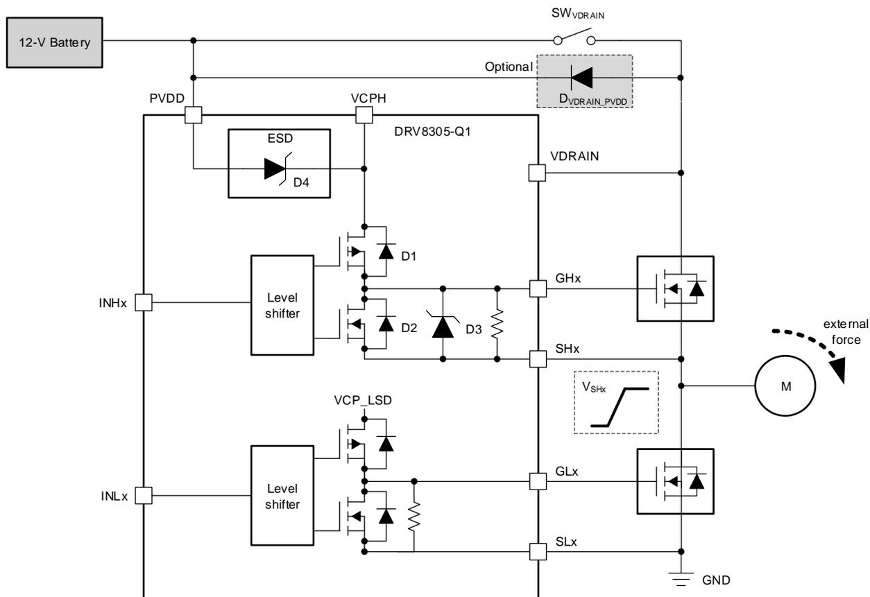
Figure 24. Power Supply Consideration in Generator Mode
