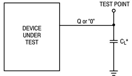
\* Includes all probe and jig capacitance.
