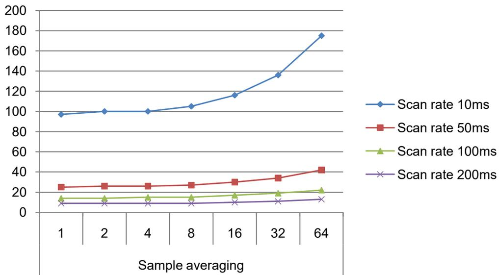
**Figure 32-9.** Power Consumption [ $\mu\text{A}$ ]
