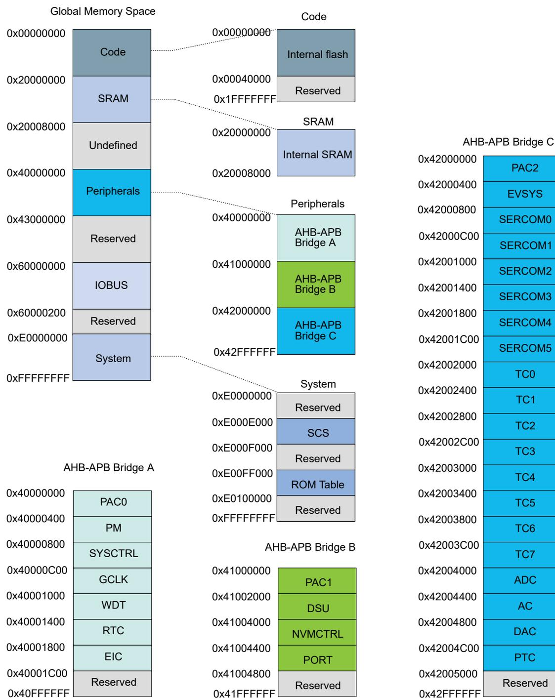
This figure represents the full configuration of the SAM D20 device with maximum flash and SRAM capabilities and a full set of peripherals. Refer to the [Configuration Summary](#) for details.
