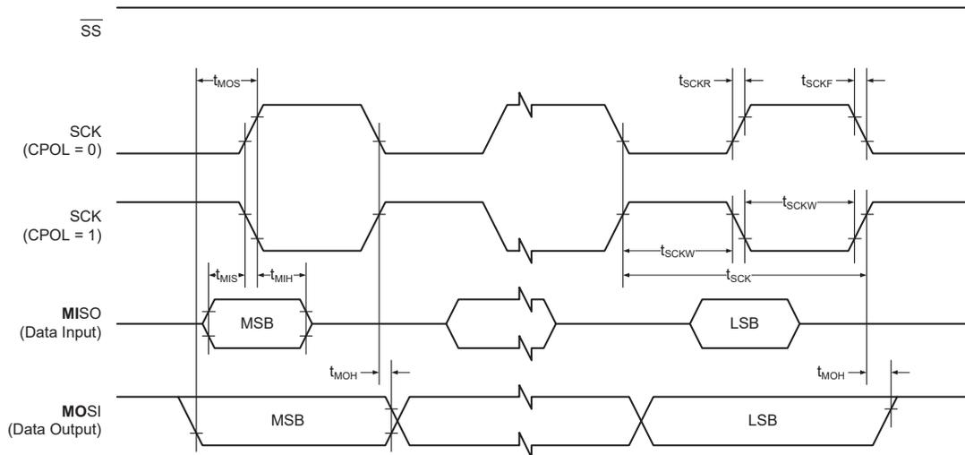
Figure 32-15. SPI timing requirements in Client mode
