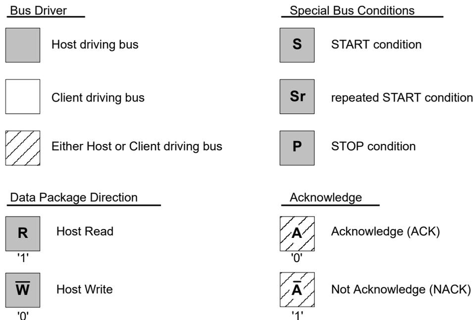
Figure 26-3. Basic I<sup>2</sup>C Transaction Diagram
