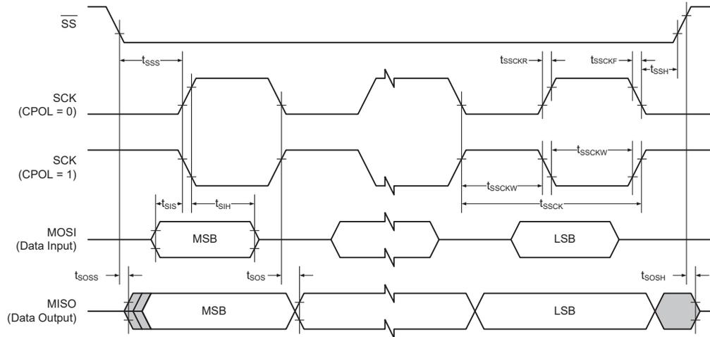
Table 32-50. SPI timing characteristics and requirements<sup>(1)</sup>
