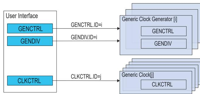
Writing these registers is done by setting the corresponding ID bit group. To read a register, the user must write the ID of the channel, *i*, in the corresponding register. The value of the register for the corresponding ID is available in the user interface by a read access.
