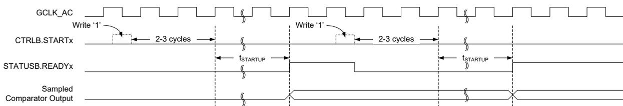
For low-power operation, event-triggered measurements can be performed during sleep modes. When the event occurs, the Power Manager will start CLK\_AC\_DIG. The comparator is enabled, and after the startup time has passed, a comparison is done and appropriate peripheral events and interrupts are also generated. The comparator and CLK\_AC\_DIG are then disabled again automatically, unless configured to wake up the system from sleep.
