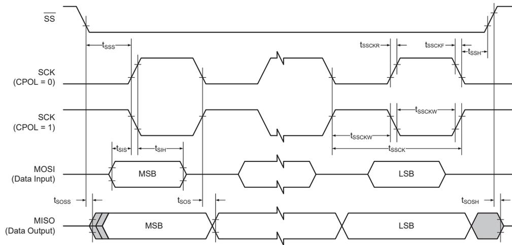
**Table 34-46. SPI Timing Characteristics and Requirements<sup>(1)</sup>**
