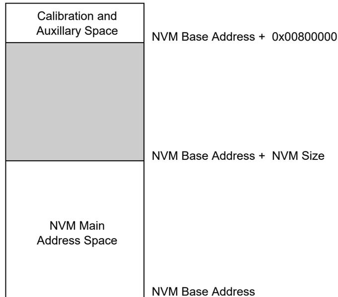
The lower rows in the NVM main address space can be allocated as a boot loader section by using the BOOTPROT fuses, and the upper rows can be allocated to EEPROM Emulation, as shown in the figure below.
