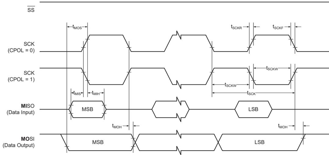
Figure 34-8. SPI Timing Requirements in Client Mode
