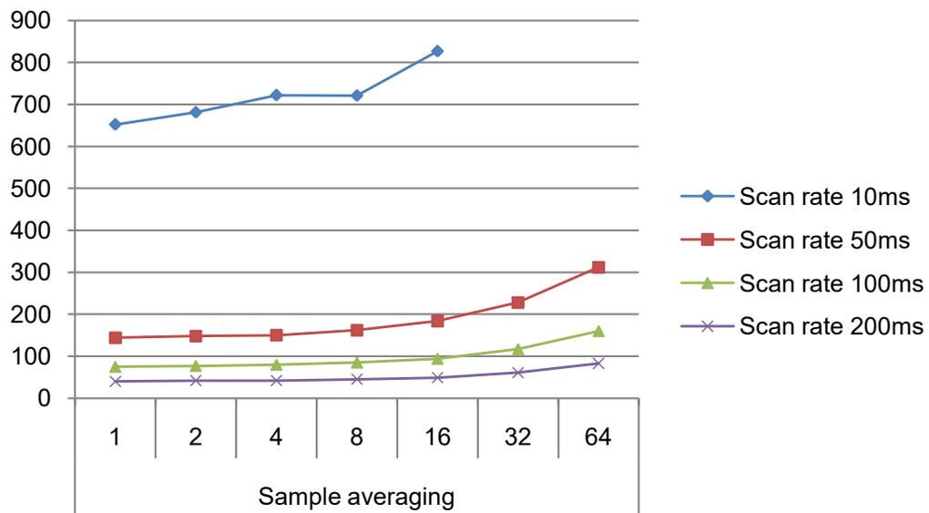
**Figure 32-11.** Power Consumption [ $\mu\text{A}$ ]
