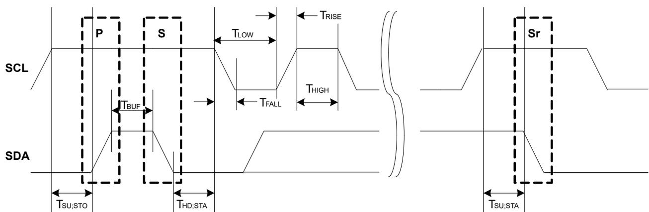
The following parameters are timed using the SCL low time period  $T_{LOW}$ . This comes from the Host Baud Rate Low bit group in the Baud Rate register (BAUD.BAUDLOW). When BAUD.BAUDLOW=0, or the Host Baud Rate bit group in the Baud Rate register (BAUD.BAUD) determines it.
