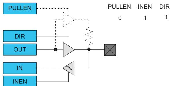
Figure 21-8. I/O Configuration - Output with Pull
