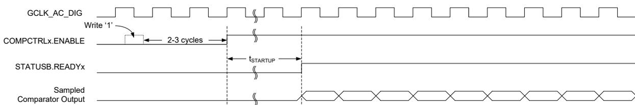
For low-power operation, comparisons can be performed during sleep modes without a clock. The comparator is enabled continuously, and changes of the comparator state are detected asynchronously. When a toggle occurs, the Power Manager will start CLK\_AC\_DIG to register
