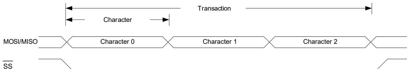
The SPI host must pull the SPI select line ( $\overline{SS}$ ) of the desired client low to initiate a transaction if multiple clients are connected to the bus. The SPI select line can be wired low if there is only one SPI client on the bus. The host and client prepare data to send via their respective Shift registers, and the host generates the serial clock on the SCK line.
