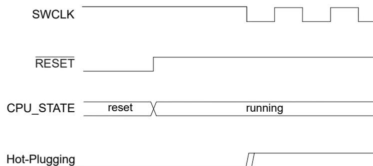
The presence of a debugger probe is detected when either Hot-Plugging or Cold-Plugging is detected. Once detected, the Debugger Present bit of the Status B register (STATUSB.DBGPRES) is set. For security reasons, Hot-Plugging is not available when the device is protected by the NVMCTRL security bit.
