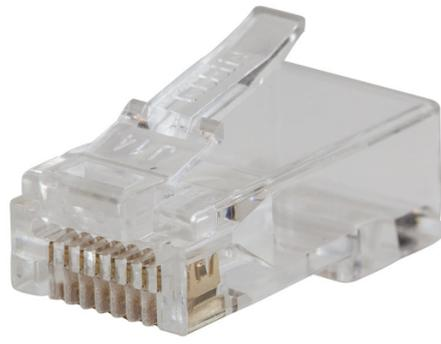
Exclusive Klein-designed Pass-Thru™ CAT5e modular plugs for fast, reliable connector installations for data applications. Cable easily passes through connector for consistent and secure termination. Saves time, trims flush to end face when used with Klein Tools Pass-Thru™ Modular Crimper VDV226-110, and eliminates wasted materials.
