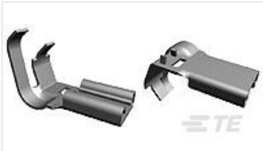
TE Part #1742626-1 250 FASTON,FLAG,REC.,16-14 AWG, NPST
