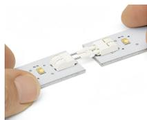
Assembly: Place PCBs on a flat surface and connect terminal blocks on adjoining PCBs via board-to-board link.
