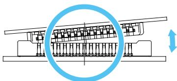
3) Do not remove the connector by pulling from the FPC corner as shown below.
