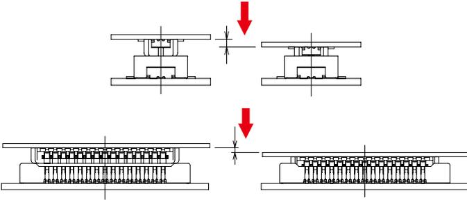
2) When fully aligned the connectors are parallel to each other with restricted longitudinal and lateral movement. Mate them parallel to each other.
