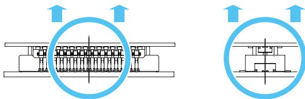
2) If the connector cannot be removed by pulling it out parallel to its mating partner, it can be removed by extracting the connector diagonally in the direction of the pitch as shown in the below figure.
