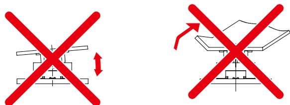
4) Insufficient FPC rigidity may result in connector breakage as shown in the below figure.
