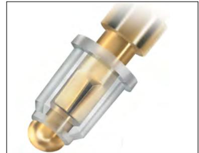
Pin receptacles can be utilized as discrete connectors for the plugging and unplugging of components on PC boards. They can be utilized individually or in random arrays where the usage is small. They can be handled and loaded manually in preparation for soldering or, with a different style shell, for press-fitting. When the requirement is for volume placement of receptacles, socket carriers or tape and reel packaging are tremendous labor-saving solutions for our customers.
