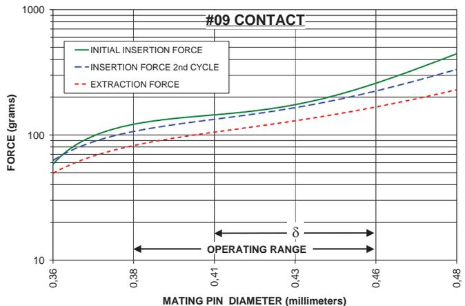
The insertion / extraction force characteristics above were derived using a 0,76 micrometers gold-plated contact and polished steel gauge pins having a bullet-shaped tip.
