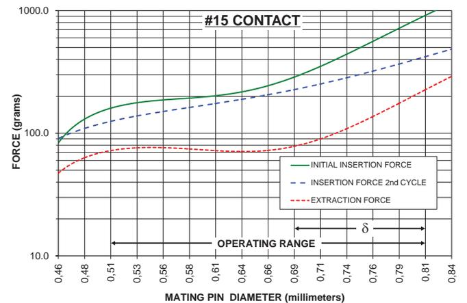
The insertion / extraction force characteristics above were derived using a 0,76 micrometers gold-plated contact and polished steel gauge pins having a bullet-shaped tip.
