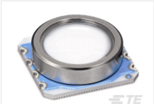
TE Part #325540009-00 MS5540-CM 1BAR WHITE GEL TUBE
