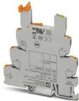
6.2 mm PLC basic terminal block for output functions with push-in connection, without relay or solid-state relay, for mounting on DIN rail NS 35/7,5, with load return line connection (BB), 1 N/O contact, input voltage 24 V AC/DC
