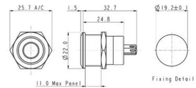
LED terminals marked + and -. Switch terminals unmarked.
