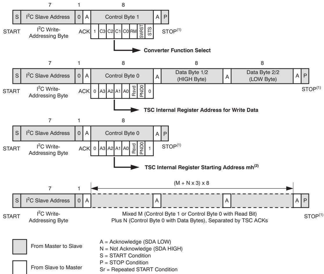
NOTES: (1) In order to start the next sequence, a STOP condition must be followed by a START condition. If no STOP is used, then a Repeated START must be used. Also note that if a STOP condition is issued in High-Speed mode, the mode will revert to the previous mode: Fast or Standard.
