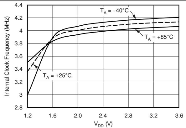
**Figure 15. Internal Oscillator Clock Frequency vs V<sub>DD</sub> Supply Voltage**
