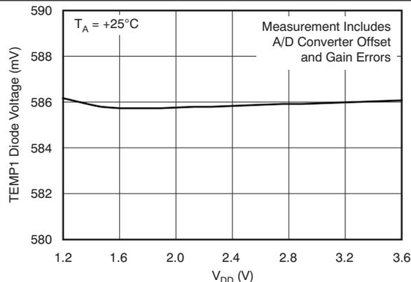
Figure 13. TEMP1 Diode Voltage vs V<sub>DD</sub> Supply Voltage
