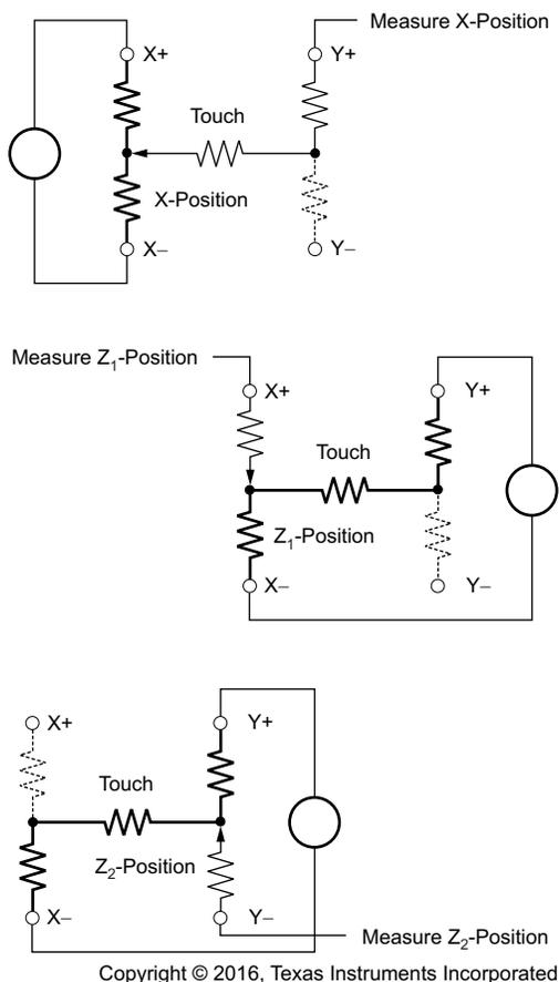
Figure 17. Pressure Measurement
