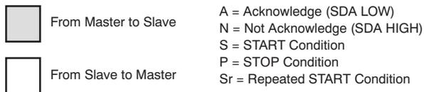
NOTES: (1) In order to start the next sequence, a STOP condition must be followed by a START condition. If no STOP is used, then a Repeated START must be used. Also note that if a STOP condition is issued in High-Speed mode, the mode will revert to the previous mode: Fast or Standard.
