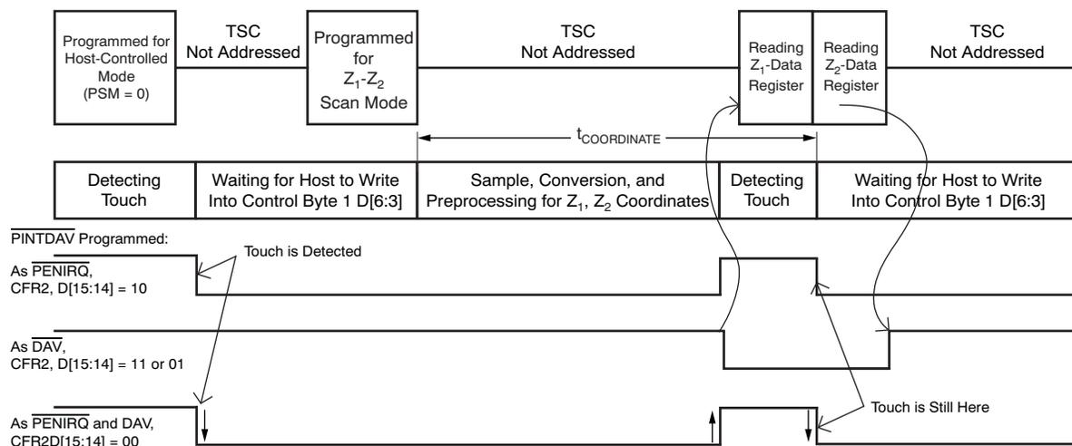
**Figure 30. Example of a Z<sub>1</sub> and Z<sub>2</sub> Coordinate Touch Screen Scan (with Panel Stabilization Time) Using TSMODE 3**
