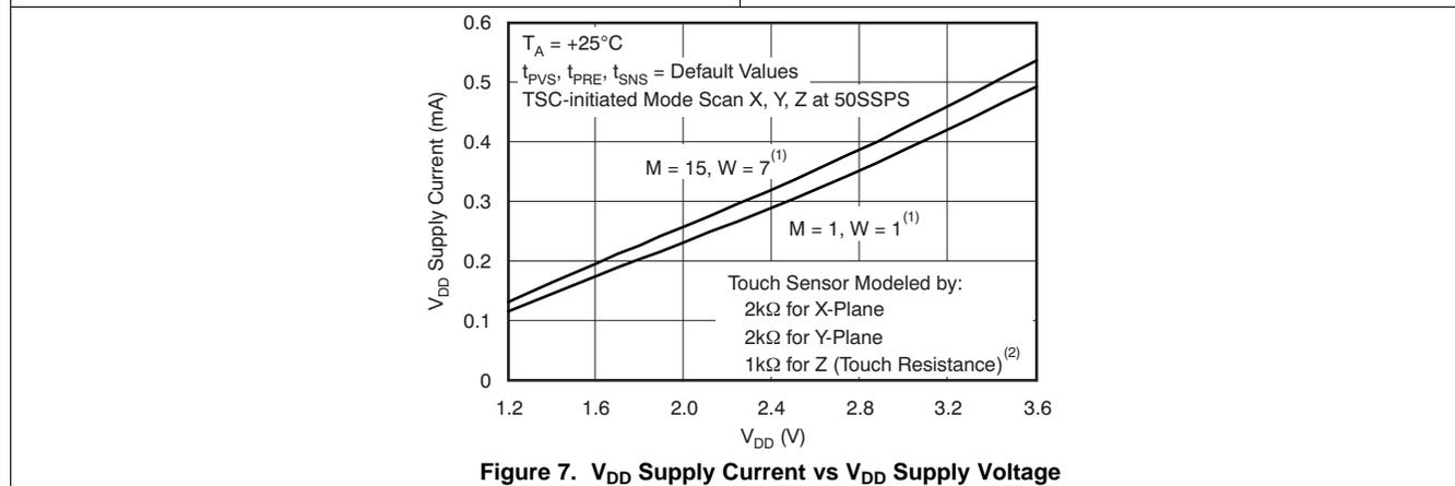
Figure 7.  $V_{DD}$  Supply Current vs  $V_{DD}$  Supply Voltage
