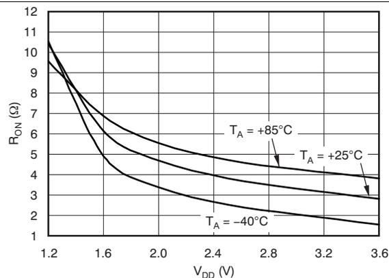
Figure 11. Switch-on Resistance (X<sub>P</sub>, Y<sub>P</sub>) vs V<sub>DD</sub> Supply Voltage
