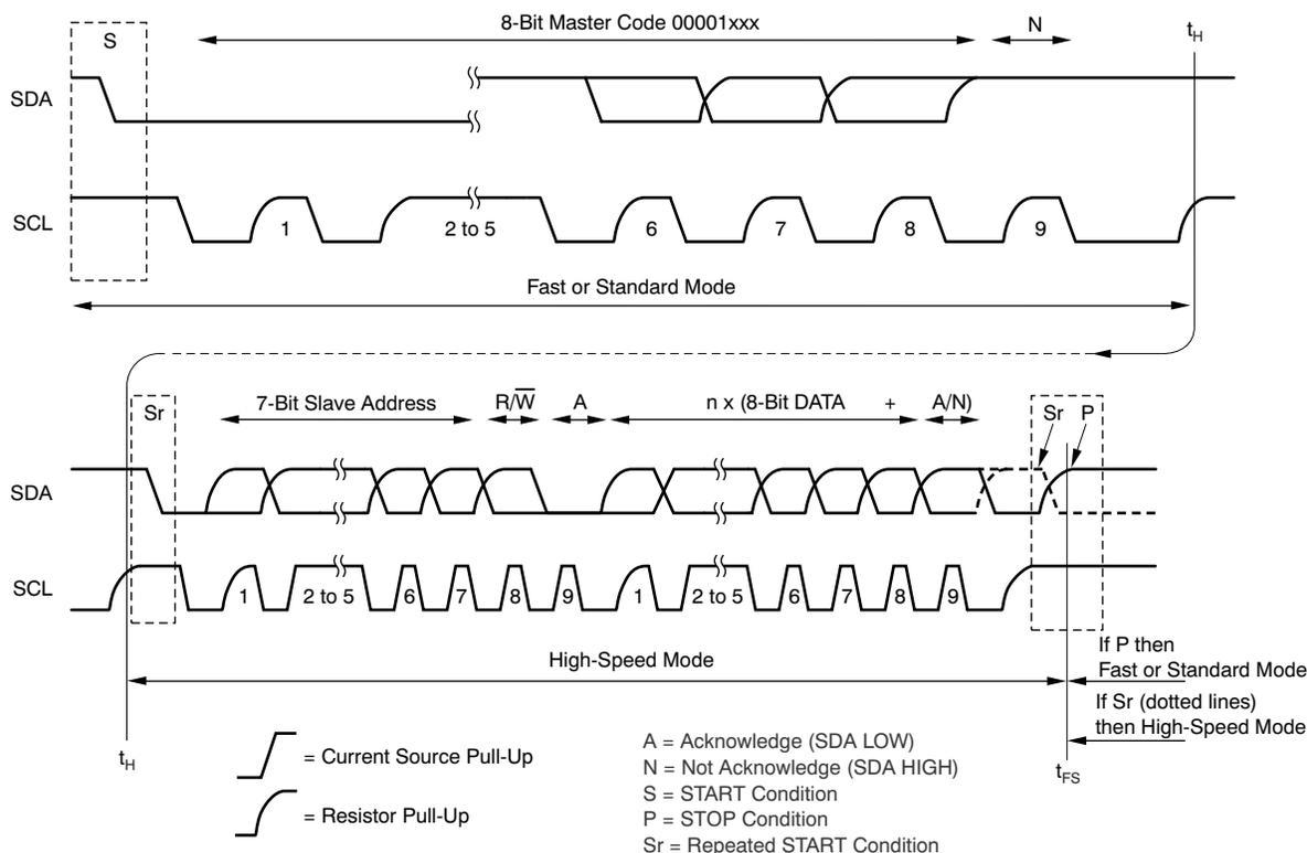
Figure 24. Complete High-Speed Mode Transfer
