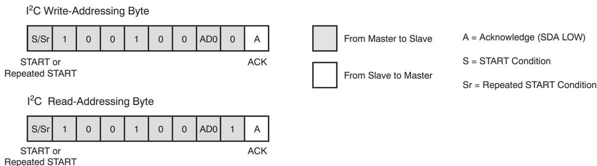
Figure 32. I<sup>2</sup>C Bus Addressing (Slave Address Byte Format)
