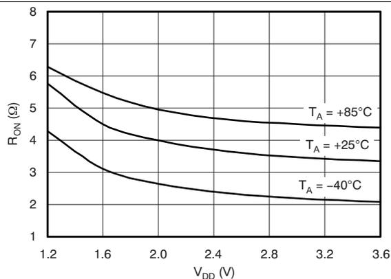
Figure 10. Switch-on Resistance (X<sub>N</sub>, Y<sub>N</sub>) vs V<sub>DD</sub> Supply Voltage
