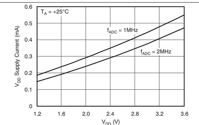
Figure 6.  $V_{DD}$  Supply Current vs  $V_{DD}$  Supply Voltage
