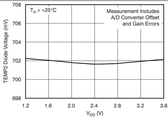
**Figure 14. TEMP2 Diode Voltage vs V<sub>DD</sub> Supply Voltage**
