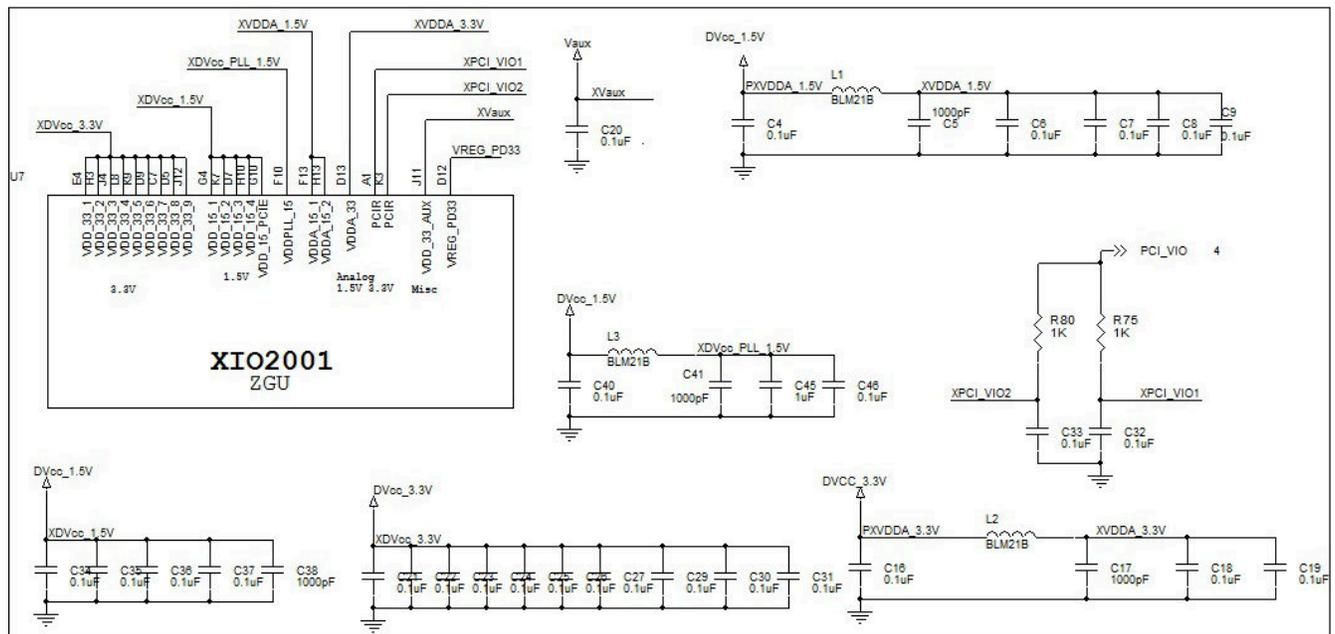
Figure 9-8. Power Filtering
