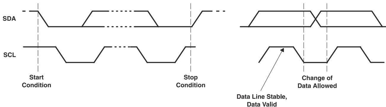
**Figure 8-10. Serial-Bus Start/Stop Conditions and Bit Transfers**
