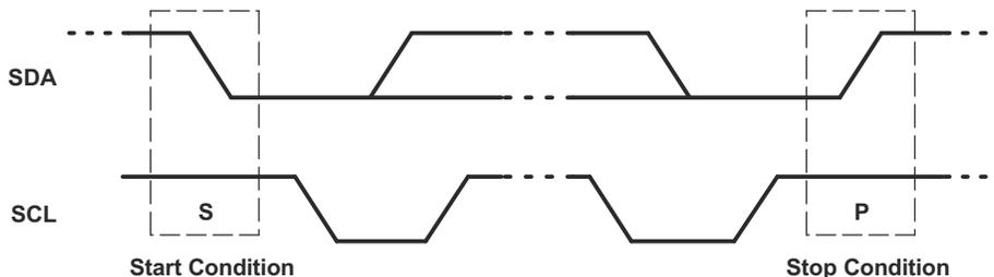
**Figure 8-2. Definition of Start and Stop Conditions**
