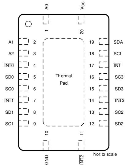
**Figure 5-2. RGY Package, VQFN (20 Pins), Top View**
