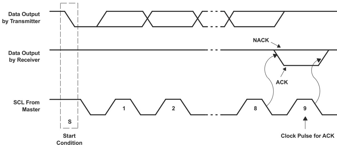
**Figure 8-4. Acknowledgment on the I<sup>2</sup>C Bus**
