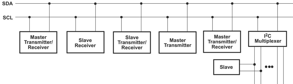
**Figure 8-3. System Configuration**
