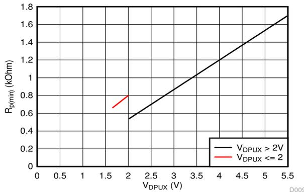
$V_{OL} = 0.2 \cdot V_{DPUX}$ ,  $I_{OL} = 2$  mA when  $V_{DPUX} \leq 2$  V
