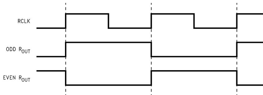
Figure 4. "Worst Case" Deserializer ICC Test Pattern
