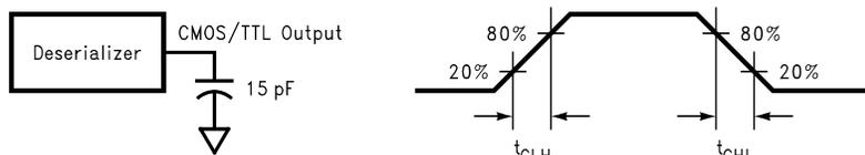
Figure 6. Deserializer CMOS/TTL Output Load and Transition Times
