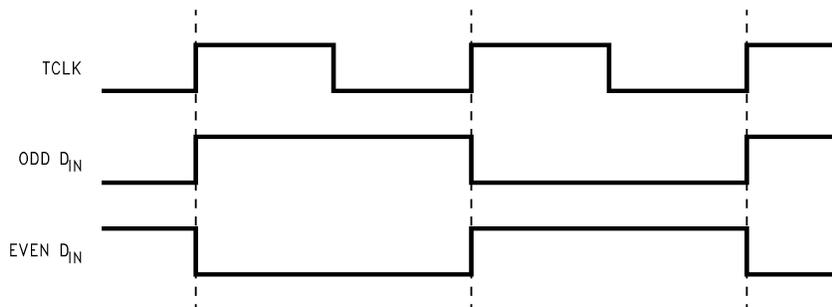
Figure 3. "Worst Case" Serializer ICC Test Pattern
