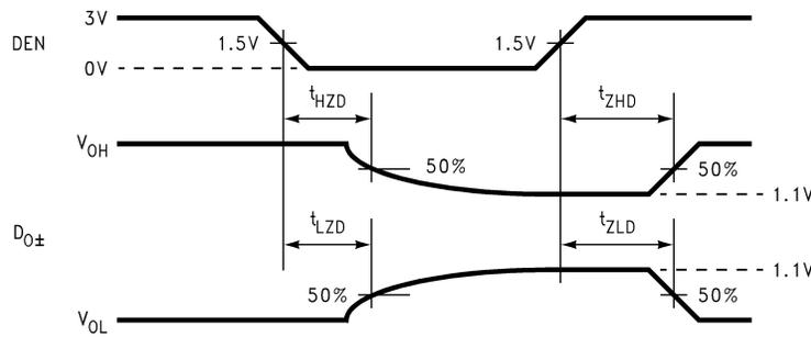
**Figure 9. Serializer Tri-state Test Circuit and Timing**
