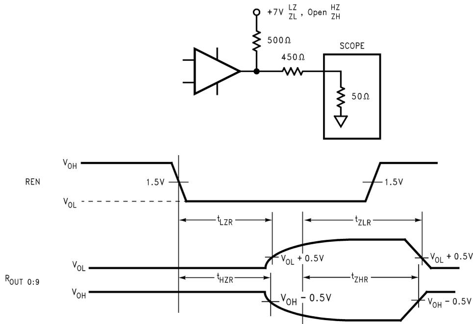
Figure 15. Deserializer Tri-state Test Circuit and Timing
