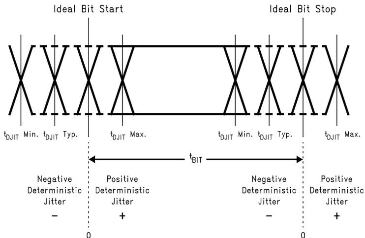
Figure 20. Deterministic Jitter and Ideal Bit Position
