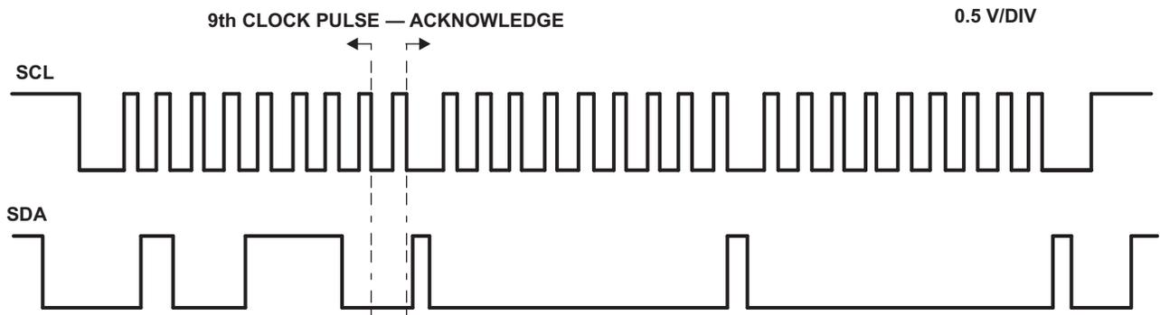
Figure 10. Bus A (0.9-V to 5.5-V Bus) Waveform
