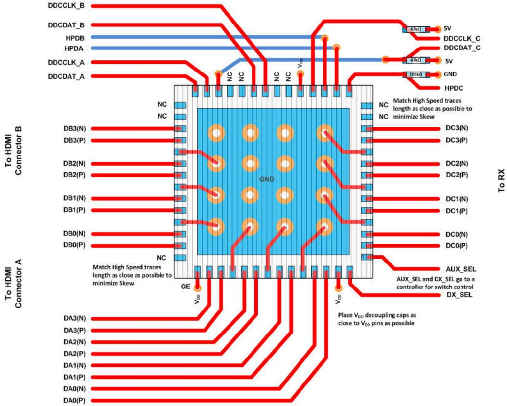
**Figure 10-3. RTQ Layout for 2:1 HDMI Sink Application**
