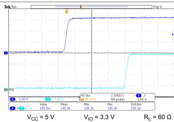
Figure 9-5.  $t_{PROP(LOOP2)}$
