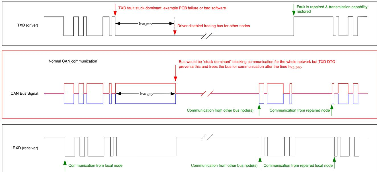
**Figure 8-2. Example Timing Diagram for TXD Dominant Timeout**
