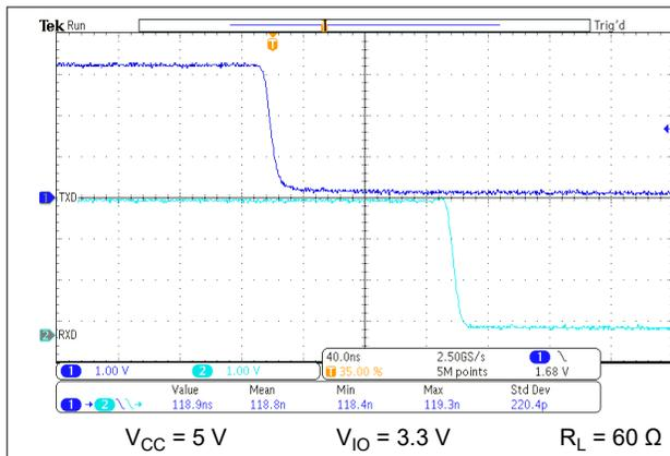
Figure 9-4.  $t_{PROP(LOOP1)}$
