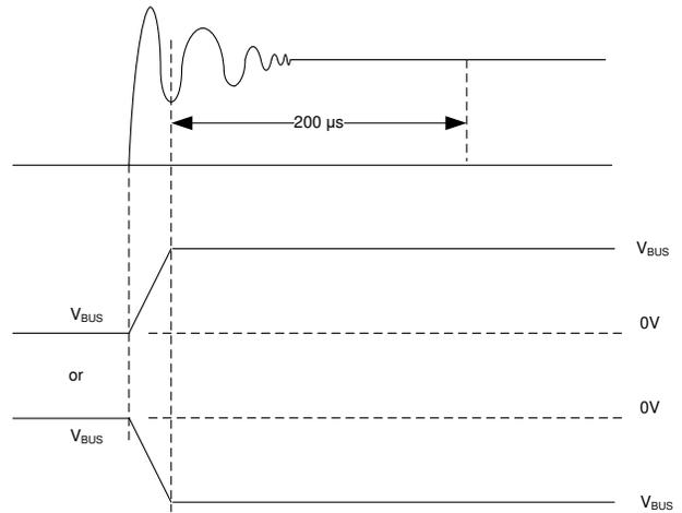
**Figure 7-7. Driver Short-Circuit Current Test and Measurement**
