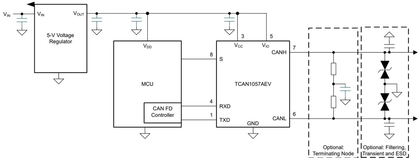
Figure 9-1. Transceiver Application Using 5 V I/O Connections
