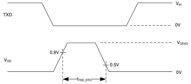
**Figure 7-6. TXD Dominant Timeout Test Circuit and Measurement**
