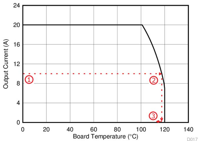
$$V_{IN} = 12 \text{ V} \quad V_{DD} = 5 \text{ V} \quad V_{OUT} = 1.8 \text{ V} \quad f_{SW} = 500 \text{ kHz} \quad L_{OUT} = 0.29 \text{ } \mu\text{H}$$
