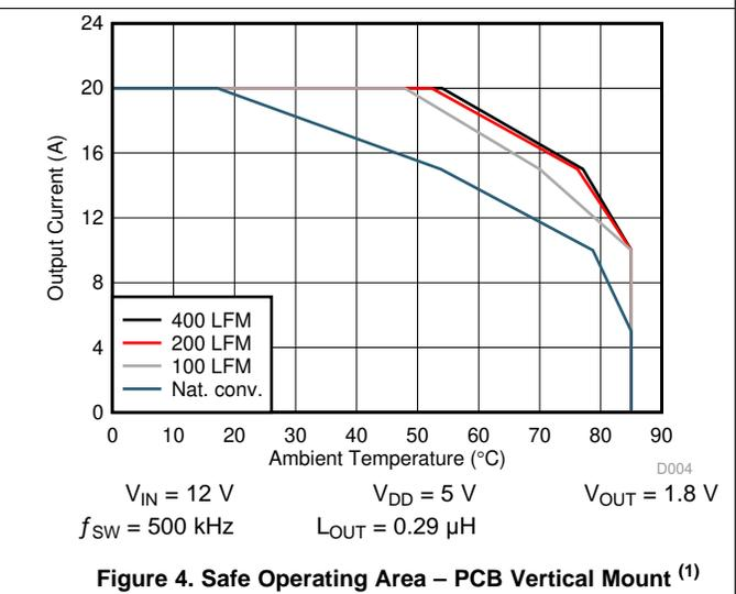
(1) The Typical CSD97376Q4M system characteristic curves are based on measurements made on a PCB design with dimensions of 4 in (W) x 3.5 in (L) x 0.062 in (T) and 6 copper layers of 1-oz copper thickness. See the [Application and Implementation](#) section for detailed explanation.
