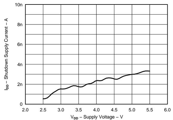
Figure 6. Shutdown Supply Current vs Supply Voltage
