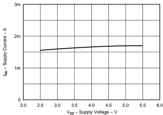
Figure 5. Supply Current vs Supply Voltage
