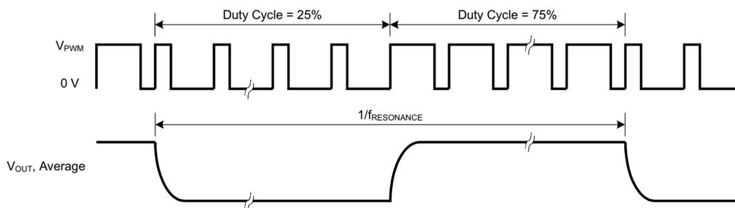
**Figure 13. LRA Example for 1/2 Full-Scale Drive**
