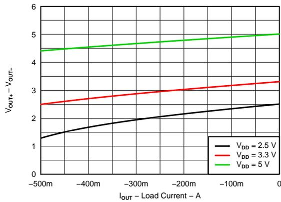
Figure 1. Output Voltage (High) vs Load Current
