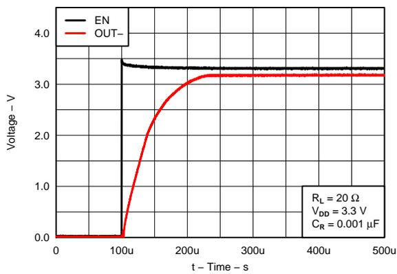
Figure 11. Startup vs Time
