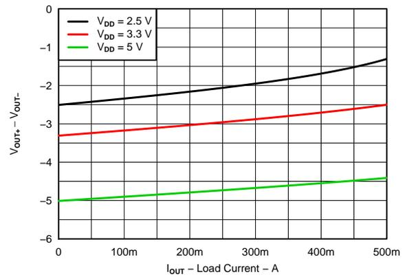
Figure 2. Output Voltage (Low) vs Load Current
