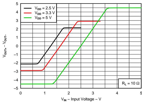
Figure 3. Output Voltage vs Input Voltage
