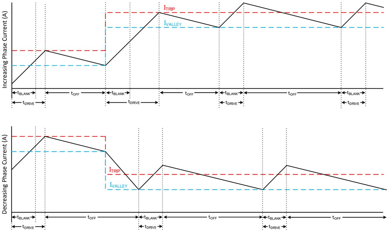
**Figure 7-13. Smart tune Ripple Control Decay Mode**
