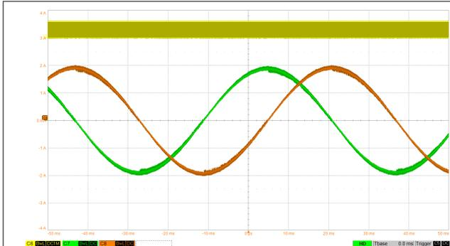
**Figure 8-7. 1/256 Microstepping With smart tune Ripple Control Decay**
