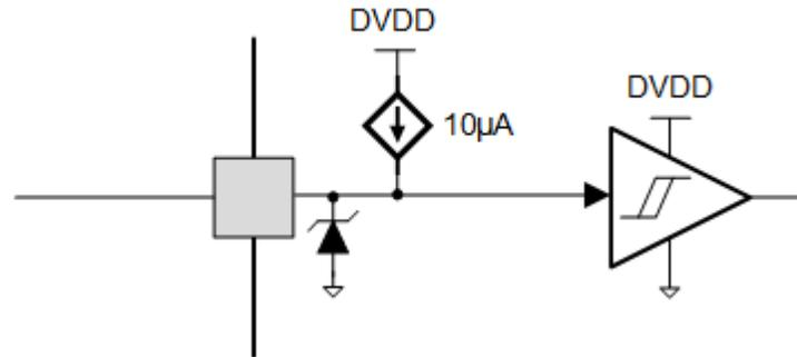
**Figure 7-17. Logic-Level with Internal Pull-up Input Pin Diagram**
