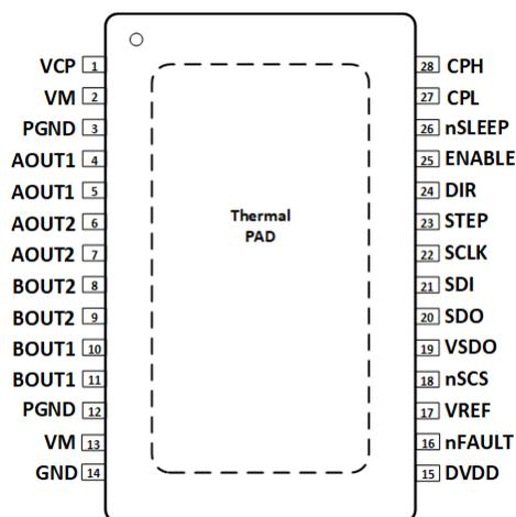
Figure 5-1. PWP PowerPAD™ Package 28-Pin HTSSOP Top View
