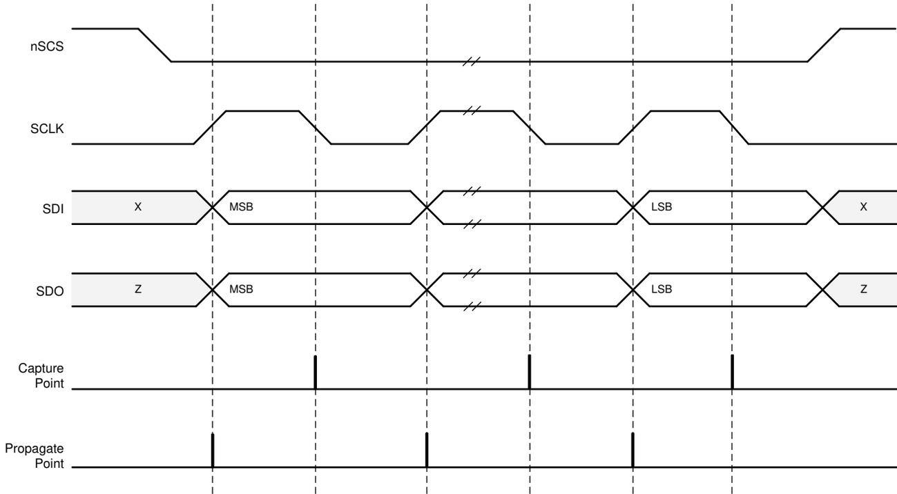
**Figure 7-29. SPI Transaction**
