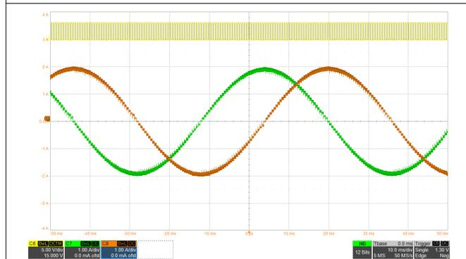
Figure 8-5. 1/32 Microstepping With smart tune Ripple Control Decay
