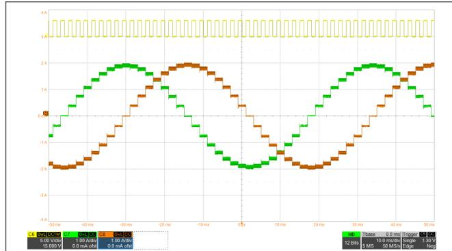
Figure 8-3. 1/8 Microstepping With smart tune Ripple Control Decay
