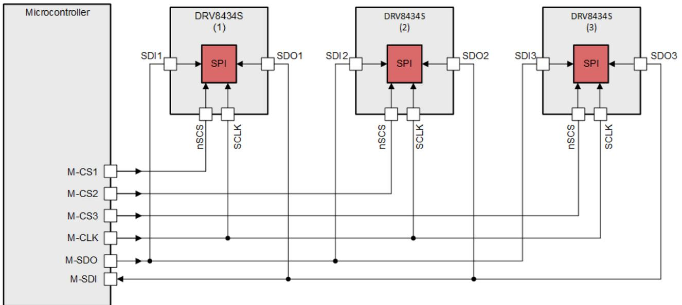
**Figure 7-30. Three DRV8434S Devices Connected in Parallel Configuration**
