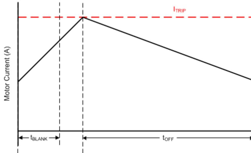
**Figure 7-5. Current Chopping Waveform**
