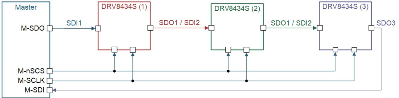
**Figure 7-24. Three DRV8434S Devices Connected in Daisy Chain**
