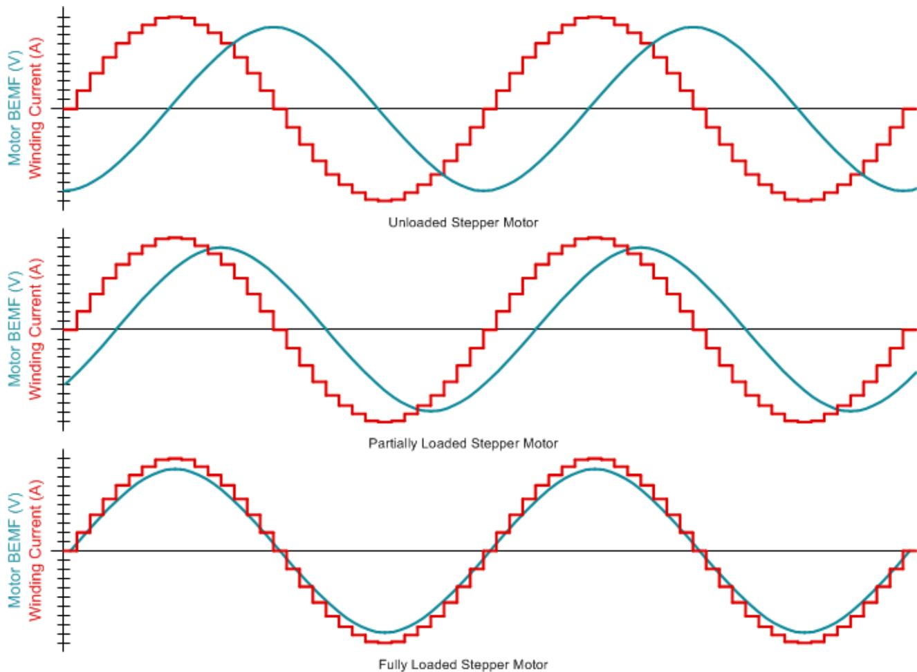
**Figure 7-21. Stall Detection by Monitoring Motor Back-EMF**
