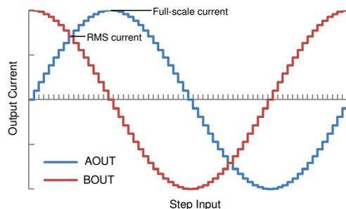
**Figure 7-1. Full-Scale and RMS Current**
