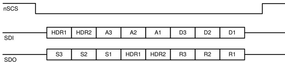
**Figure 7-26. SPI Data Sequence for Three Devices**
