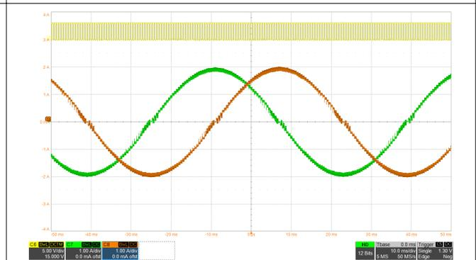
Figure 8-6. 1/32 Microstepping With smart tune Dynamic Decay
