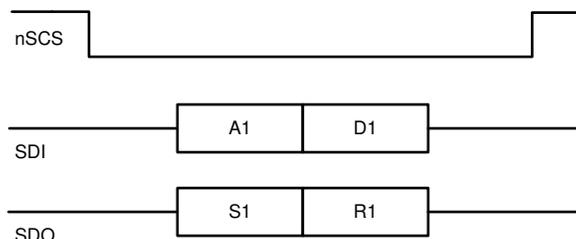
**Figure 7-23. SPI Transaction Between MCU and the device**
