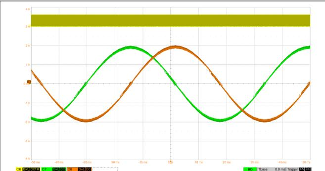
**Figure 8-8. 1/256 Microstepping With smart tune Dynamic Decay**
