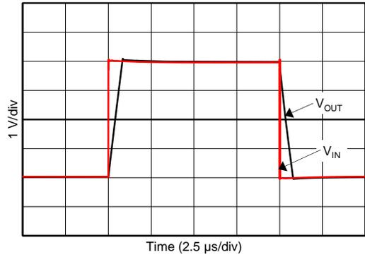
$V_{IN} = 4\text{ V}_{PP}$ ,  $G = +1$ ,  $C_L = 15\text{ pF}$
