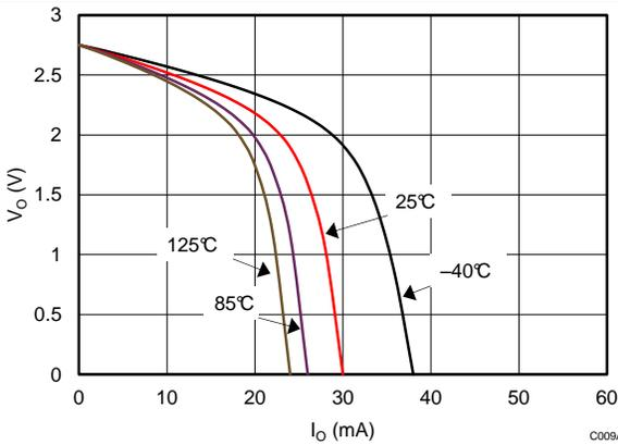
Figure 15. Output Voltage Swing (Positive) vs Output Current
