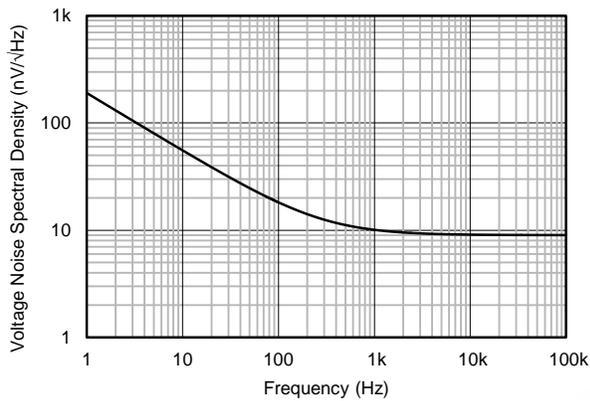
Figure 21. Input Voltage Noise Spectral Density vs Frequency
