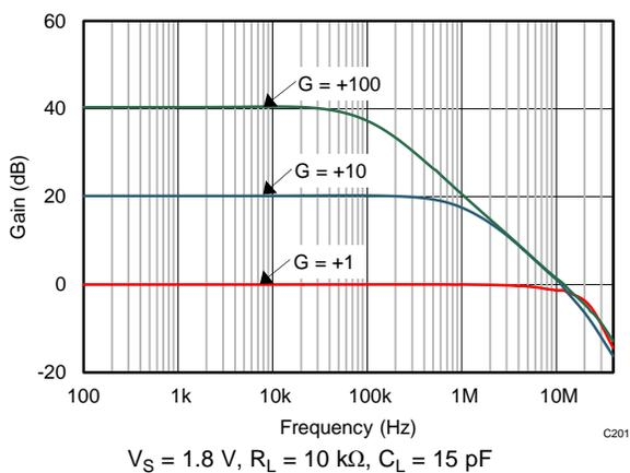
Figure 23. Closed-Loop Gain vs Frequency
