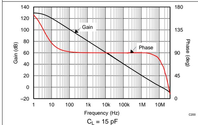
Figure 5. Open-Loop Gain and Phase vs Frequency
