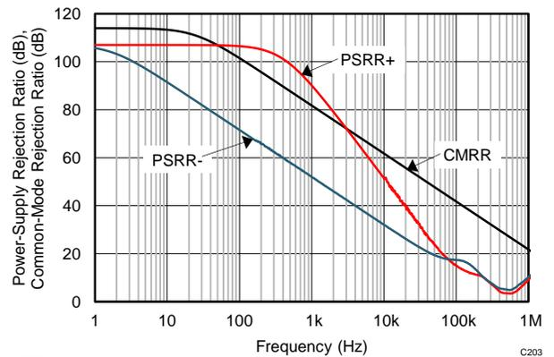
Figure 18. CMRR and PSRR vs Frequency
