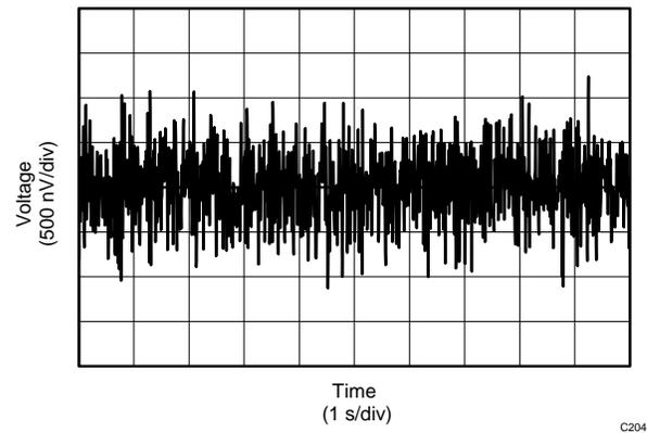
Figure 22. 0.1-Hz to 10-Hz Input Voltage Noise
