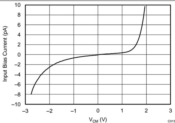
Figure 11. Input Bias Current vs Common-Mode Voltage
