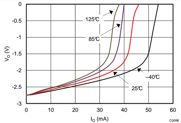
Figure 16. Output Voltage Swing (Negative) vs Output Current
