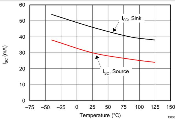
Figure 17. Short-Circuit Current vs Temperature
