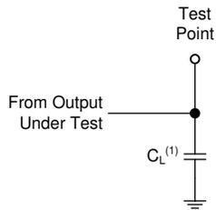
1. Includes probe and test-fixture capacitance.
