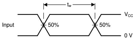
**Figure 6-2. Voltage Waveforms, Standard CMOS Inputs Pulse Duration**
