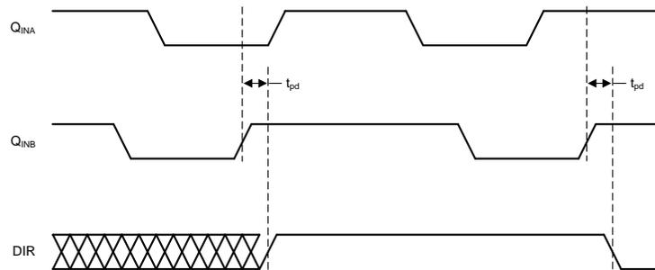
Figure 8. Timing Diagram for Quadrature Encoder Application
